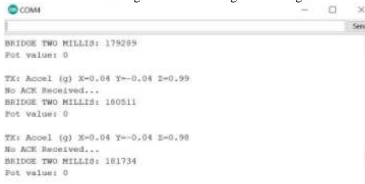
Fig. 2 Serial Monitor of Transmitting Module on Bridge 2 showing values being transmitted
