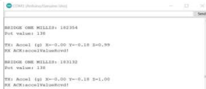
Fig. 1 Serial Monitor of Transmitting Module on Bridge 1 showing values being transmitted
